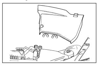
2. Remove side cover by pulling up on front of cover.
